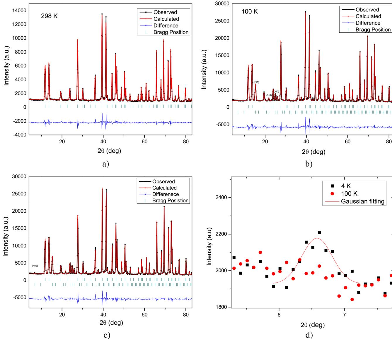
**Figure 4.** Rietveld refinement of the neutron powder diffraction data at (a) 298 K, (b) 100 K, and (c) 4 K. (d) Comparison of 4 and 100 K neutron data at low  $2\theta$ , showing (100) peak at 4 K.
