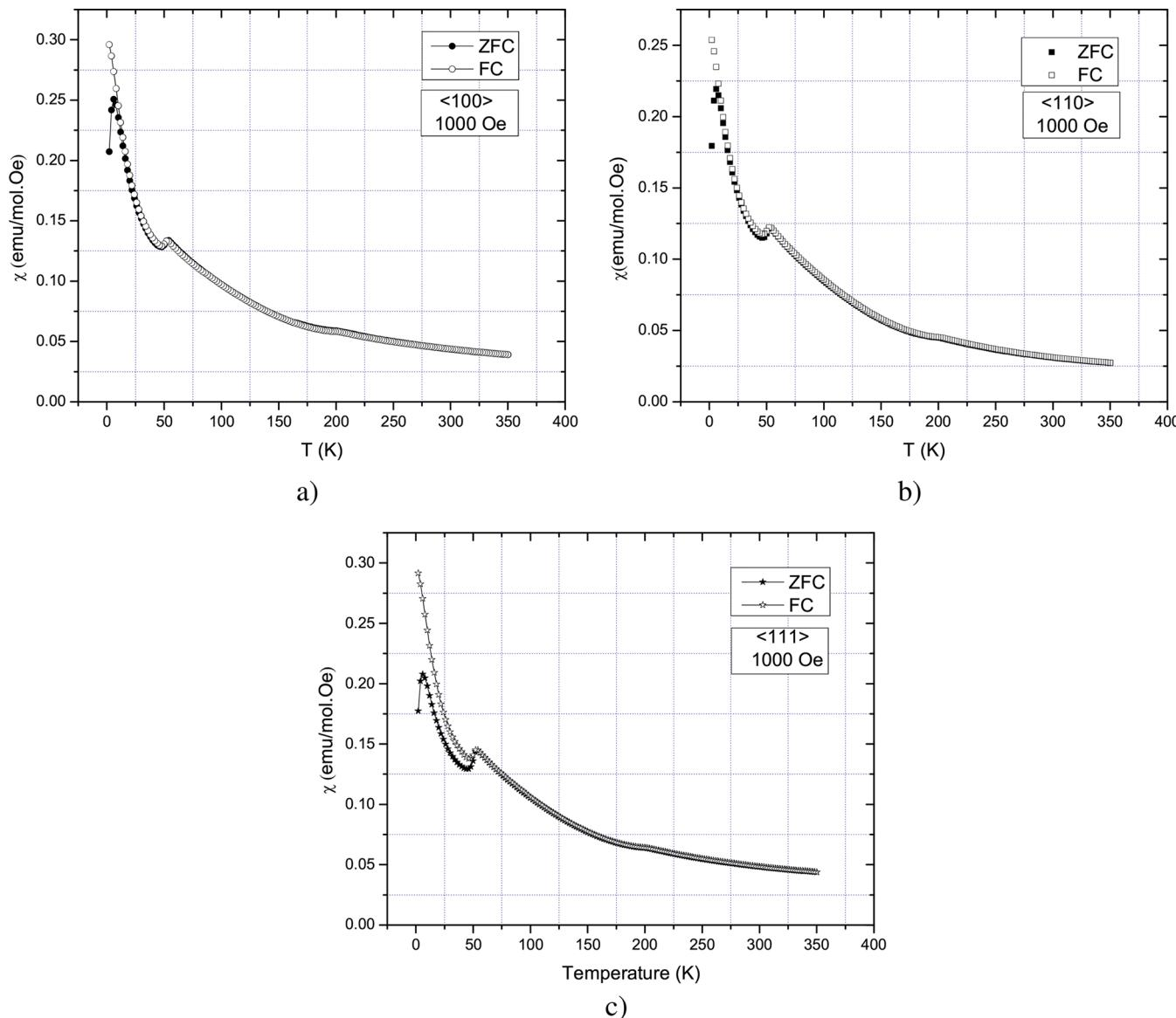
Figure 1. (a) ZFC-FC magnetic susceptibility of  $\text{Mn}_6\text{Ni}_{16}\text{Si}_7$  crystal at 1000 Oe field applied along (a)  $\langle 100 \rangle$ , (b)  $\langle 110 \rangle$ , and (c)  $\langle 111 \rangle$ .
