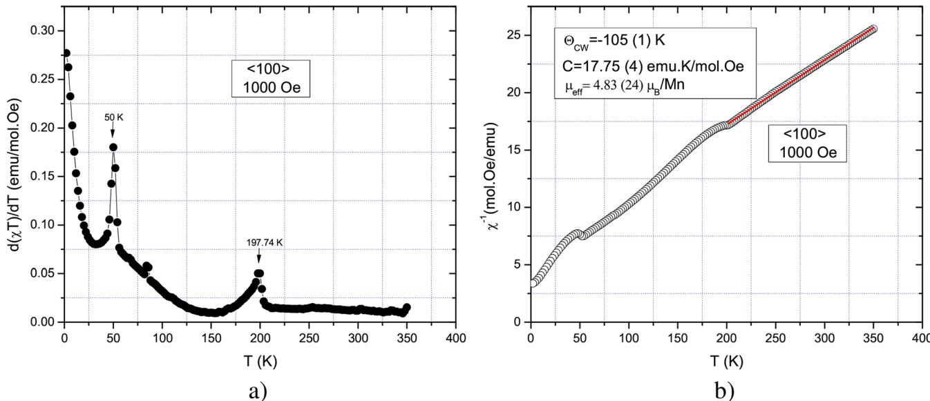
**Figure 2.** (a) FC  $d(\chi T)/dT$  vs  $T$  plot identifying the transition temperatures, for crystal with the applied field along the  $\langle 100 \rangle$  direction. (b) Curie–Weiss fit on the inverse susceptibility data of  $Mn_6Ni_{16}Si_7$  single crystals along  $\langle 100 \rangle$  above 200 K.
