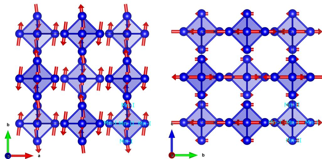
Figure 7. Hidden spin-canted antiferromagnetic structure is favored at 4 K. The two-dimensional magnetic symmetry is broken, and the moments are canted in  $(ab)$  plane. Magnetic moment vectors are guide to eye only. The structures presented in the figure corresponds to projection along the (a)  $ab$  and (b)  $bc$  planes, respectively.
